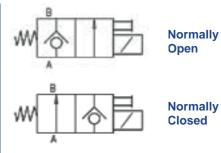
N.B. On the VAS 1 1/4" Ported Valve the closed path is B to A port, Not A to B port!
